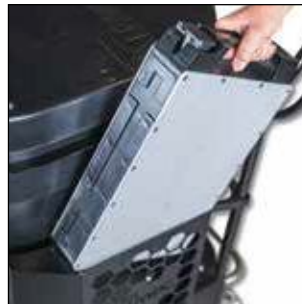
Insert the new battery directly
